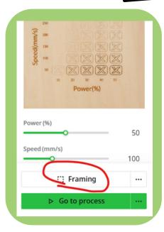
Once our Power, Speed and Pass is set, we can move on to Framing. Framing moves the crosshair around to preview where the very edges of your design will land on your material. This step is very simple!
